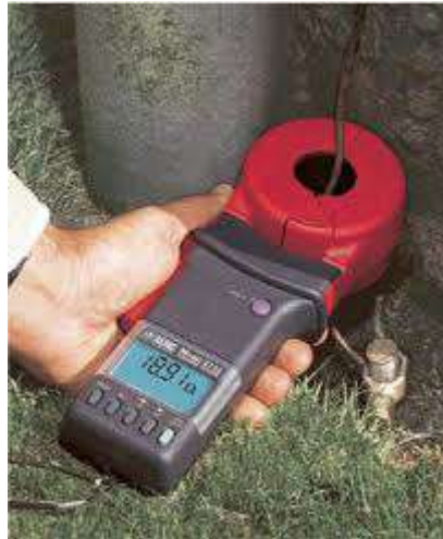
Fig.4 Clamp on method earth resistance
